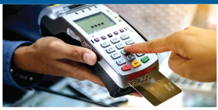
electronic fund transfers. The terminal facilitates transactions by allowing the merchant or their client to swipe, insert or hold a card near the device to capture information and confirm payments.
